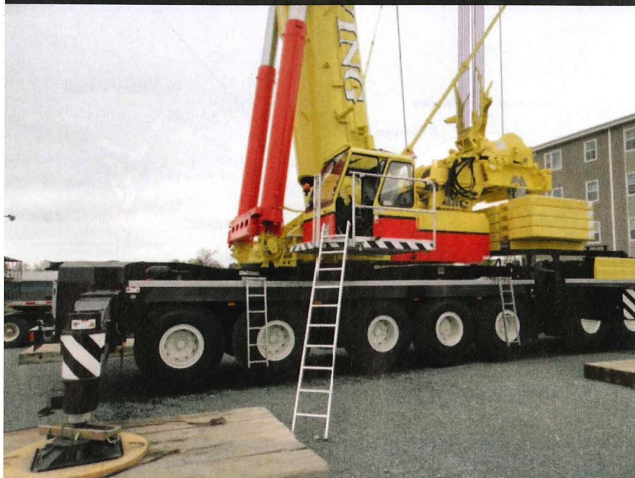
A large mobile crane that has been nano-coated for ocean shipment.
