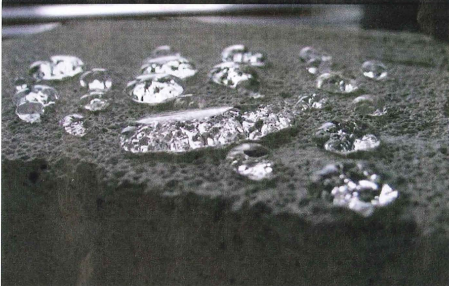
Water droplets on a concrete surface exhibiting high contact angles.
