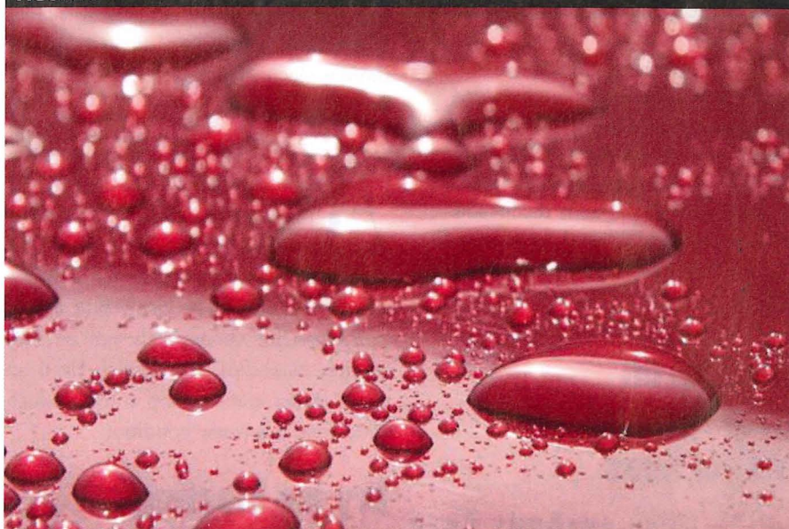
Water droplets on a metal surface exhibiting high contact angles.
